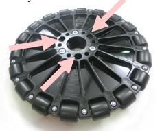
Step 2: Press in a 1614ZZ <sup>3</sup>/<sub>8</sub>" id bearing to the top off the first wheel, and to the bottom of the second omni wheel.
