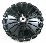
Step 3: Place the second omni wheel above it. Align the holes so that the three #10-32 x 2-1/4" SHCS will go into the holes that have the arrows on them. Insert and tighten in three #10-32 x 2-1/4" SHCS with the cordless drill. Make sure the rollers are alternating.
